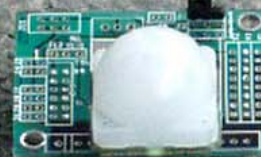
PIR: Passive InfraRed motion detector
