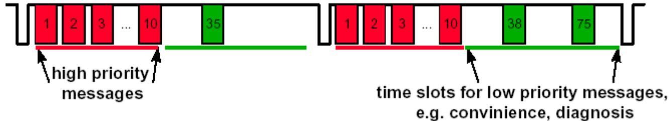
**Slots with fixed priorities are reserved for synchronous messages. These slots are assigned in every cycle (1-10) and allow a deterministic analysis of message latencies.**
