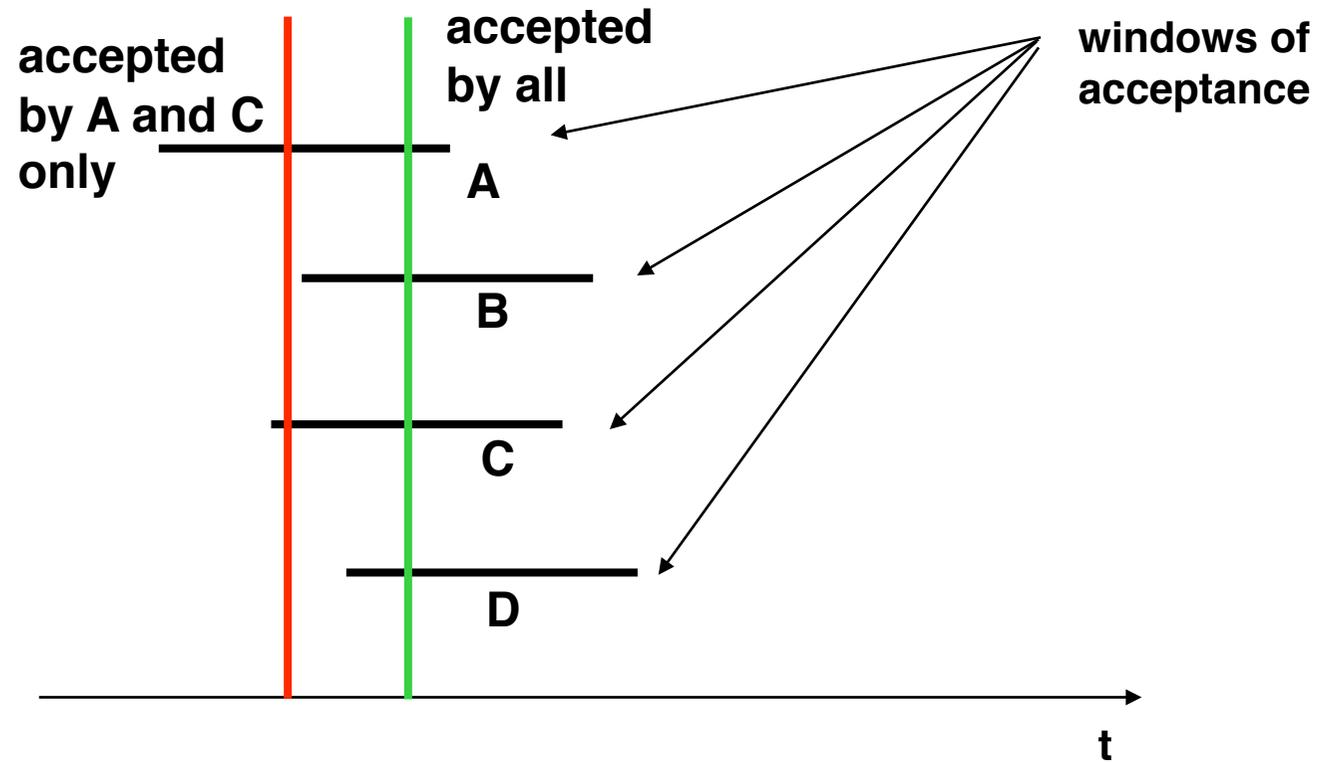
Slightly-off-specification failures can occur at the interface between the analog and the digital world.
