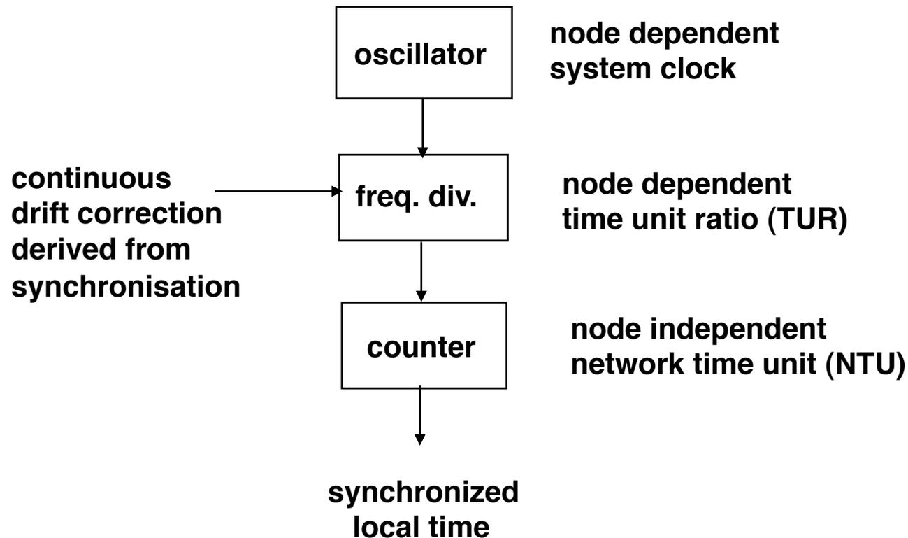
**Synchronization based on the existence of a Time Master.**
