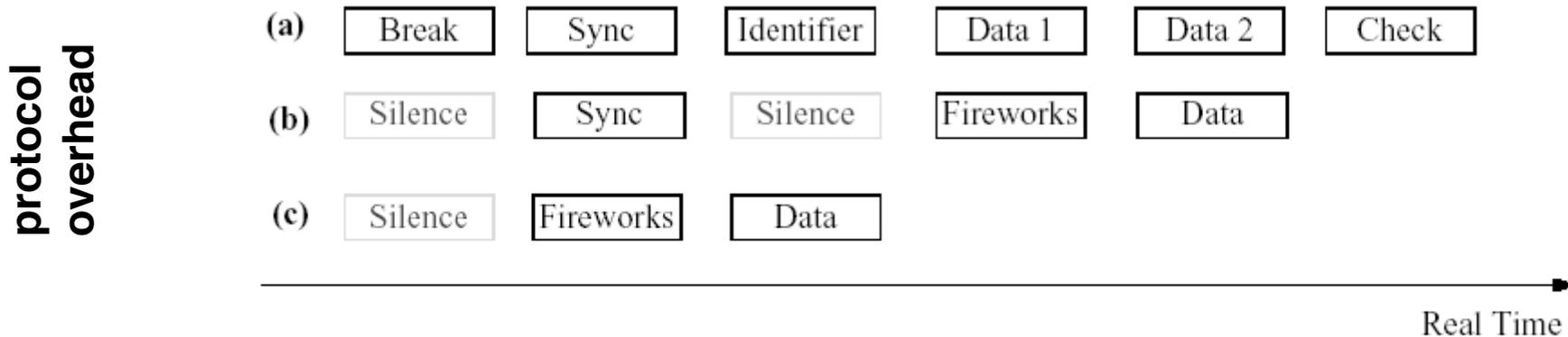
**Figure 5:** Byte Sequence of the simplest message in LIN (a), in TTP/A with start-up synchronization (b) and in TTP/A without start-up synchronization (c).
