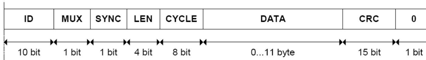
**ID:** Identifier, 10 Bit, value range: (1 ... 1023), defines the slot position in the static segment and the priority in the dynamic segment. A low ID defines a high priority. ID = 0 is reserved for the SYNC-symbol. An identifier must be unique in the network, i.e. two identical IDs would lead to a collision. Every node may use one or more identifiers in the static and the dynamic segment.
